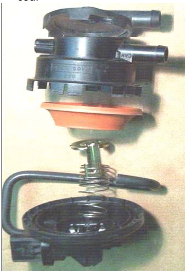
LEAK DETECTION PUMP
